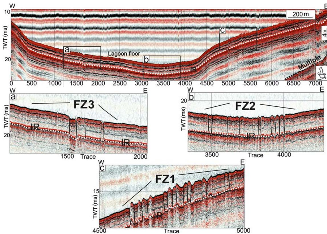
**Fig. 6** Active faults (FZ1, FZ2, and FZ3) identified along an E–W seismic profile from the middle part of the lagoon. **a** Blow-up of the FZ3 fault zone located in the western part of the lagoon. **b** Blow-up of the FZ2 fault zone located in the middle of the lagoon. **c** Blow-up of the FZ1
