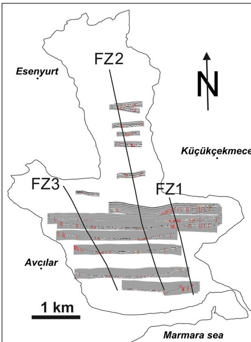
seismic profiles are clearly aligned in a general NW–SE direction. They are interpreted as representing strike-slip fault systems that may be associated with the northern branch of the NAFZ.
