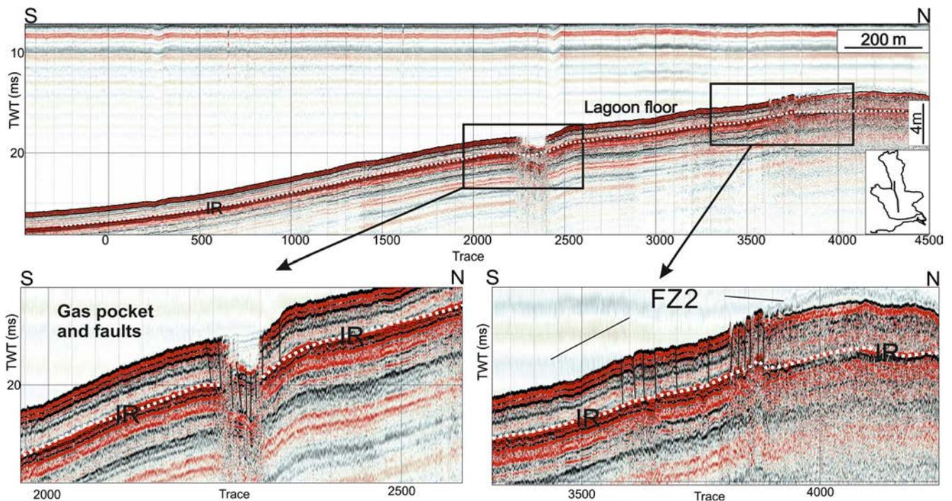
**Fig. 5** N–S-oriented seismic profile from the western lagoon area showing the location of probable gas pockets in relation to the FZ2 active fault zone. From the white dashed line (*IR*) downward, the internal sedimentary structures are masked by reverberation sections
