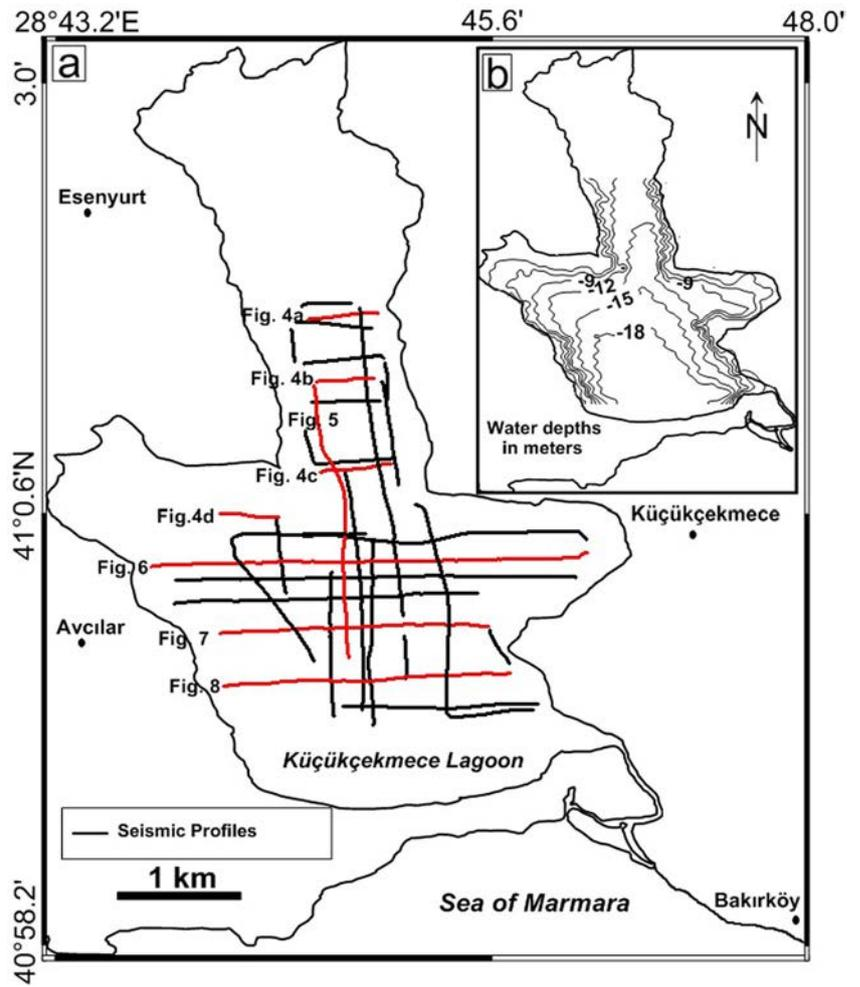
**Fig. 4** Active FZ2 (a–c) and FZ3 (d) fault zones identified on seismic profiles from the northern and western parts of the lagoon, respectively
